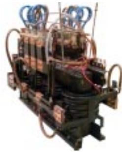
Water cooled rectifier-transformer
